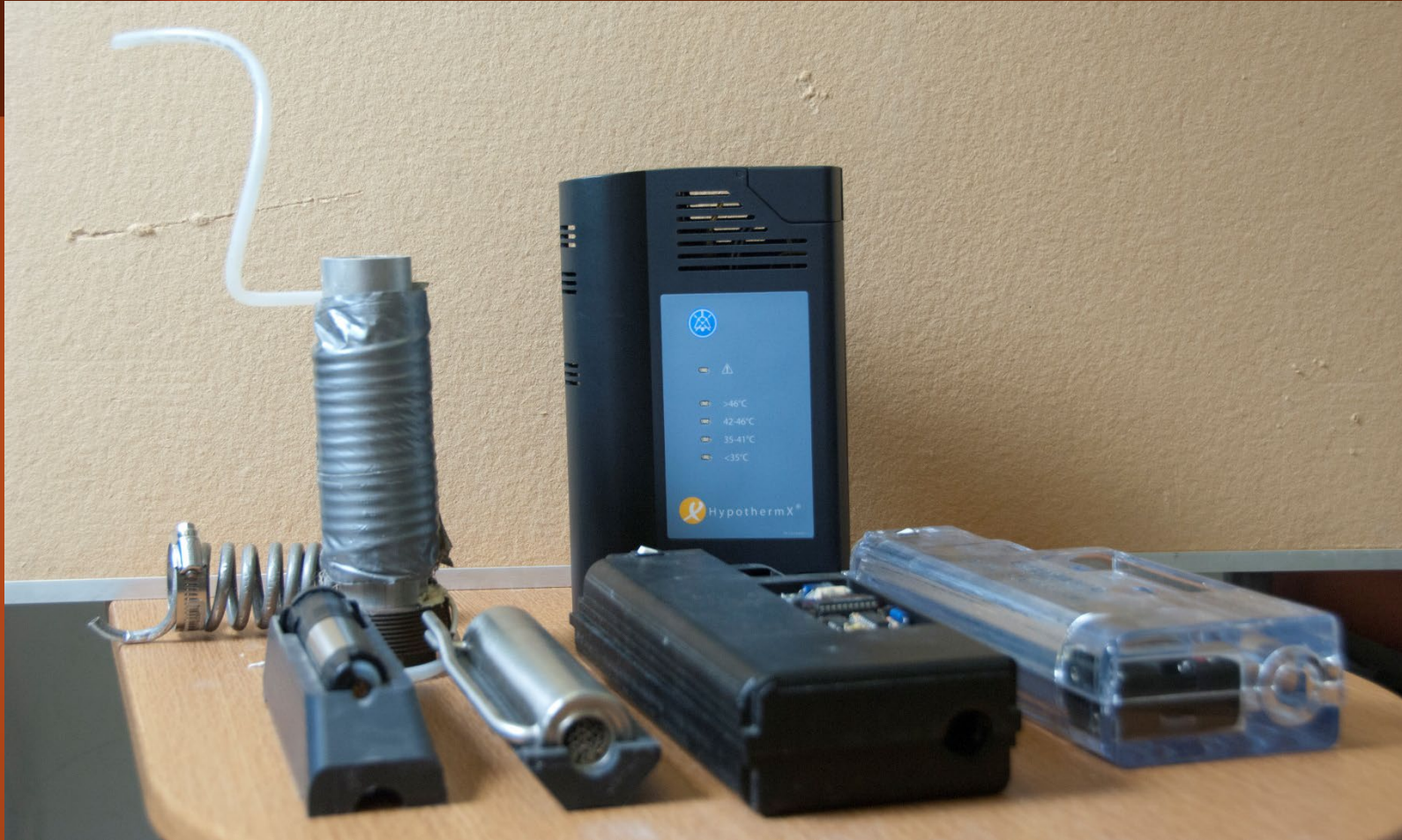
Various fluid warmer prototypes over the years, from research prototype to FDA approved product for sale
